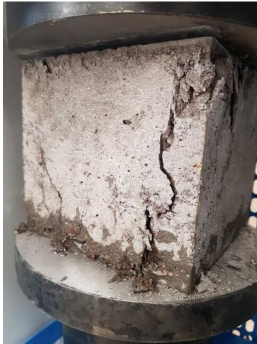
Figure 3. Failure of a concrete specimen
